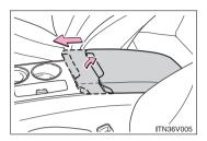
If necessary, the console box lid can slide forward. Pull the lid forward while pulling up the lever.
