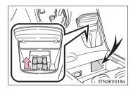
The auxiliary boxes of the front console are provided with a hole that allows cables to be passed from the power outlet and AUX adapter.
