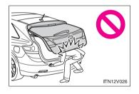
1 The back door may fall if it is not opened fully. It is more difficult to open or close the back door on an incline than on a level surface, so beware of the back door unexpectedly opening or closing by itself. Make sure that the back door is fully open and secure before using the luggage compartment.
